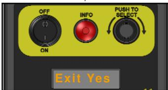
The control box will now display "Exit Yes" or by turning the "PUSH TO SELECT" knob anti clockwise "Exit No" Turning back will display "Exit Yes" again.
