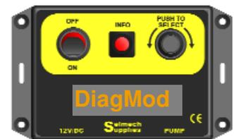
Press and release the “PRESS TO SELECT” as per diag mode but continue to hold until Diag++ is displayed.
