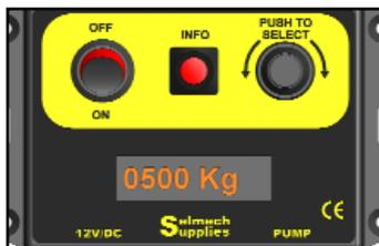
Press the "PUSH TO SELECT" knob to display the bale weight in Kg. Rotating the knob allows to enter your bale weight between 0100 Kg and 2000 Kg.
