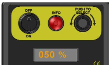
Rotating the "PUSH TO SELECT" knob will increase and decrease the percentage drive to the motor (000 to 100) this in turn increases and decreases the output of the pump.
