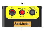
Keep holding down the "PUSH TO SELECT" Knob. until the display shows "SetModel". then release the "PUSH TO SELECT" Knob.
