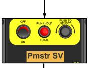
The control box will now display the current model selected. At this point by turning the PRESS TO SELECT knob, clockwise and anti clockwise, you can change model. It is strongly recommended not to change the model, unless specifically told to, as this would change the current calibration that is used for this applicator. *The model options are:* -
