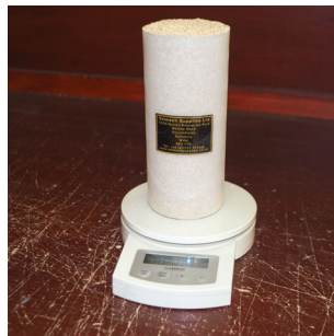
Place filled container on scales
