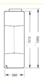
Selmech can also supply a 400 litre tank to be used in conjunction with a Dflow pump module.
