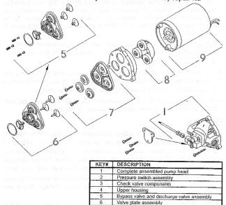
Diaphragm and piston Drive assembly Motor assembly (less
