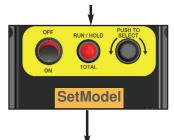
Keep holding down the "PUSH TO SELECT" Knob. until the display shows "SetModel". then release the "PUSH TO SELECT" Knob.
